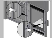
Slide the two spacers sideways away from the intermediate glass panel. The spacers stay fitted on the door.
