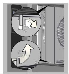
Use the tool to release the fasteners, top and bottom.
