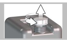
Remove the cap from the ConvoCare rinse aid mixing canister.
