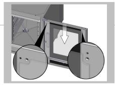
Make sure you fit the intermediate glass panel the correct way round. The two notches in the intermediate glass panel face upwards and have a different contour.
