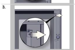
Push on the spring clip on the top right bracket and pivot the interior glass panel slightly out of the bracket.
