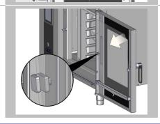
Pivot the top of the intermediate glass panel slightly away from the door; the spacers at the side are pulled slightly out of the door in the process.
