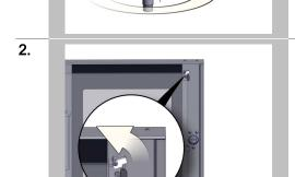
Rotate upwards the catch for the interior glass panel on the top right bracket.
