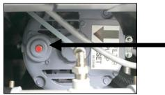
Filter Pump Reset Switch
