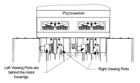
The optimum burn is a bright orange-red glow. If a blue flame is observed, or if there are dark spots on a burner face, adjust the air gas mixture as follows: On the side of the blower housing opposite the motor is a plate with a locking nut. Loosen the nut enough to allow the plate to be moved, then adjust the position of the plate to open or close the air intake opening until a bright orange-red glow is obtained. Carefully hold the plate in position and tighten the locking nut.
