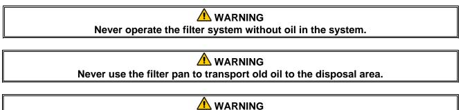
Never drain water into the filter pan. Water will damage the filter pump.
