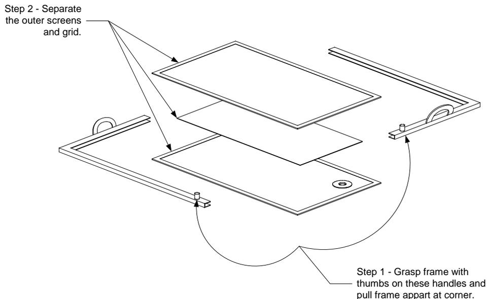
2. Separate the outer screens and grid.
