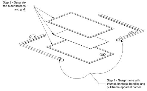
2. Separate the outer screens and grid.
