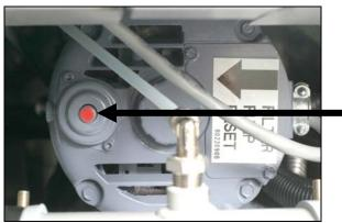
Filter Pump Reset Switch
