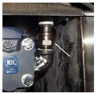
Remove hose fitting (arrow) with an open-end wrench. Use pipe sealant when installing new hose.
