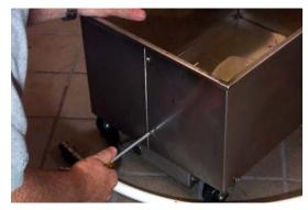
Remove screws securing outer panels.
