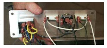
Mark wiring locations on defective switch/light before disconnecting wires.
