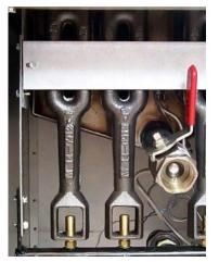
Typical frypot drain valve (SM40 shown).
