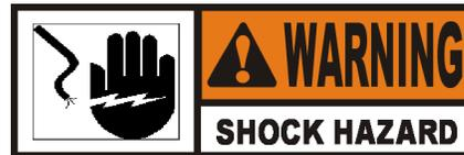
**To avoid electrical shock, the cabinet must be adequately and safely grounded (earthed) according to local electrical codes.**
