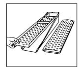
Insert columnating plate so the step goes under the lip of the finger housing and the plate lies flush with the housing side edge.
