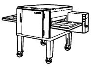
Remove the oven from the dolly and set it on the stand. The control panel should be on the right rear as you face the oven. Be sure that the oven sets squarely on the stand and is fully seated. For a single oven, install top. For double, see step 3.
