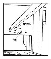
4. Before installing the retaining brackets in the oven(s), be sure all of the packing material is removed from the plenum shroud. Install the finger retaining brackets by placing them upside down and hooking the retaining pin as shown above.
