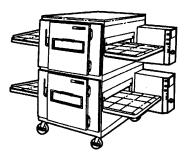
If you purchased a double stack oven, place the second oven on top of the first one. Be sure that it sets on squarely and is fully seated. The control panel goes on the right rear. Now install oven top.
