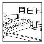
Insert assembled finger through door opening starting with lower left. NOTE: The customer MUST tell you what position to place the assembled finger in, for their application.
