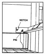
5. Rotate the finger brackets until the notches in the brackets sit on the retaining pins.
