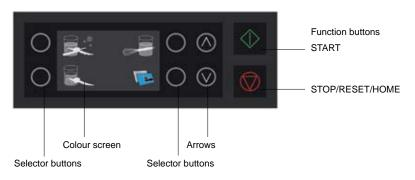
The PACOJET 2 control panel has two function buttons: START and STOP/ RESET/HOME. It also features a high resolution colour screen, four selector buttons for display functions and two buttons with arrows for increasing and decreasing settings. The following sections describe these in greater detail.
