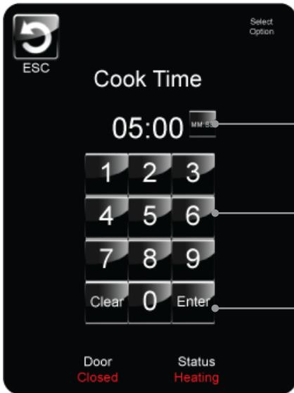
Touch to toggle between minutes and seconds (MM:SS) and hours and minutes (HH:MM).
