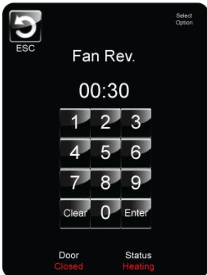
Use numeric keypad to input new fan reverse time.
