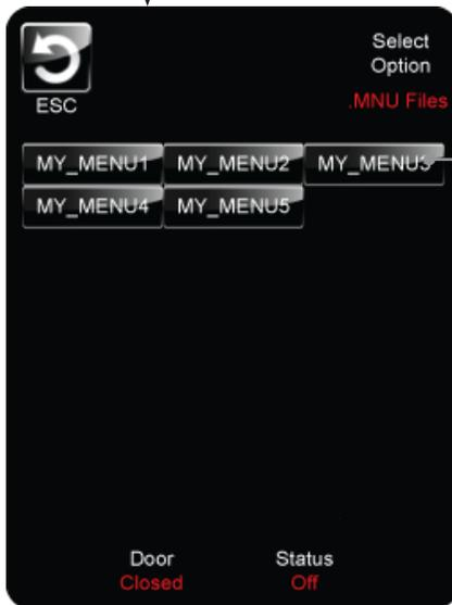
Display shows menus loaded to the thumb drive. Touch a menu name to load it to the oven.
