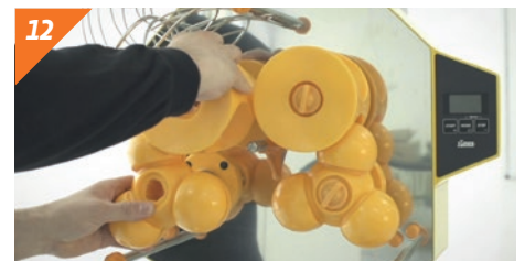
12 Take off the pressing units in pairs.
