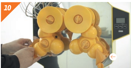
10 Pull off the peel ejectors.
